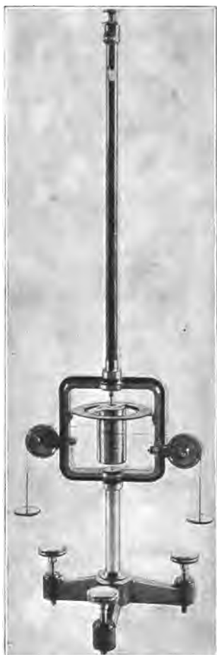
Fig. 41. Apparatus for measuring Modulus of Rigidity by the torsion of wires.
